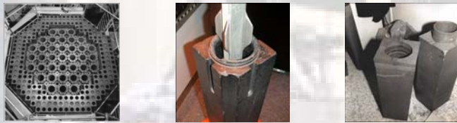
Photographs of a AGR graphite reactor core and moderator graphite bricks.
